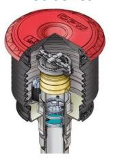
OPW and Pomeco Spill Containment Manholes are designed to prevent spilled product from entering the soil near the fill and vapor return riser connections on underground storage tanks during normal tank filling operation, or in the event of tank overfill. The spill containers catch spillage to help prevent soil contamination and groundwater pollution. OPW Thread-On Spill Containment Manholes are generally used on new tank or riser pipe installations.
