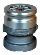
The OPW 1611AV and 1611AVB are poppeted adaptors, designed to mate with a vapor recovery elbow, for returning gasoline vapor to the tank truck during a fuel delivery to an underground tank.
