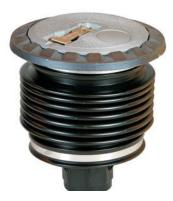
Similar to the 1-2100 Series, but has a sealable cover. The operation of the cover is similar to that of a "plumbers plug." When the lever is latched down, the plates are drawn together, expanding the seal against the machined mounting ring wall.
