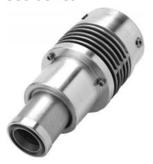
The diffuser is attached to the end of a drop tube to reduce turbulence and vapor loss during fuel fills. It also acts as a rag catcher.
