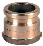
The 61SA Swivel Adaptor mates with 4" topseal delivery elbows and features a top section that rotates with hose movement while the bottom section remains securely in place maintaining seal integrity.
