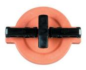
The OPW 1711T Vapor Recovery Cap is for use with the OPW 1611AV, 61VSA, 1611AVB and the 1611VR Adaptors. The 1711T is installed on the vapor recovery adaptor, when not in use, to prevent vapors from escaping and to prevent water, dust and debris from entering the tank.
